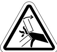
Pinch/Crush points created during assembly.
